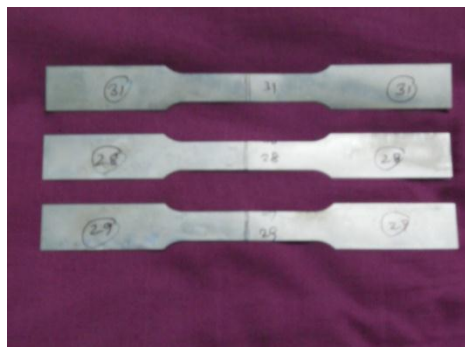
Figure 10. Tensile specimens before testing
